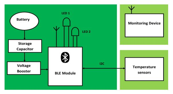
All the modules used in the solution are FCC pre- certified so that the client saves time in the pre-certification process. We designed the hardware, including schematic capture, logic design, PCB Design, EMI and EMC, i2c temperature sensor interfacing, and embedded firmware development was done in parallel to ensure on time delivery of the solution. Basic electrical testing and functional & application testing was also done to check for errors before delivery of the product.
